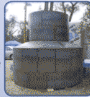
(The mold to cast 3, 6, 8, and 10 cubic meter digesters)
